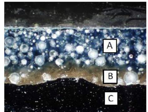
Figure 1 - Cross section of glass-fused-to-steel (enameled) tank panel. Layer A is glass frit layer, Layer B is the molecularly fused layer and layer C is the steel panel substrate.
